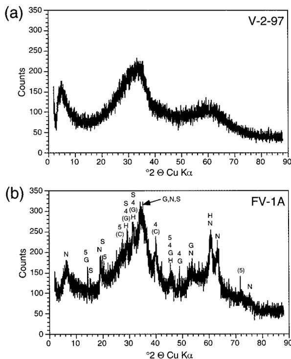
**FIGURE 3. Diffractometer patterns for sample V-2-97 (a) and FV-1A (b). The two patterns clearly demonstrate the increasing crystallinity with increasing age. V-2-97 contains only protoferrihydrite, whereas in FV-1A several sharp peaks are superimposed on top of the typical protoferrihydrite pattern: N: smectite (nontronite), G: gypsum, C: claudetite, S: scorodite, H: hematite, 4: As<sub>2</sub>O<sub>4</sub>, and 5: As<sub>2</sub>O<sub>5</sub>. Letters in brackets indicate doubtful peaks.**
