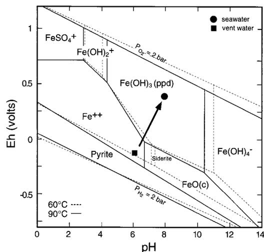
FIGURE 5. Eh-pH diagram for the system Fe-O-H-SO<sub>4</sub>-HCO<sub>3</sub> at 60 °C (dashed lines) and 90 °C (solid lines) at a pressure of 2.026 bar. Activities of Fe, SO<sub>4</sub>, and HCO<sub>3</sub> are assumed to be 10<sup>-5</sup>, 10<sup>-3</sup>, and 10<sup>-3</sup>, respectively. Fe(OH)<sub>3</sub>(ppd) is the field of amorphous Fe(III) oxyhydroxide. The arrow indicates the mixing trend between hydrothermal fluid and seawater.
