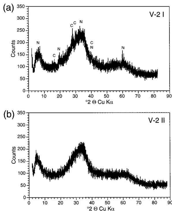
FIGURE 4. Diffractometer patterns for sample V-2 II (a) and V-2 I (b). The two patterns clearly demonstrate the importance of seawater contact during aging. The sample V-2 I, although slightly younger than V-2 II, is more crystalline because it remained in contact with either seawater or a mixture of seawater and vent fluid (seawater  $\gg$  vent fluid). C: claudetite, N: smectite (nontronite).
