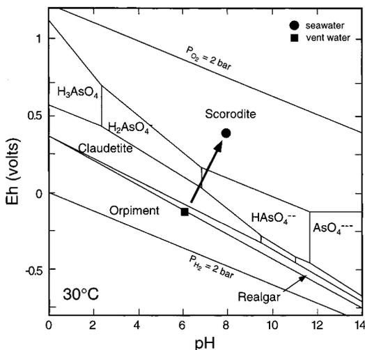
FIGURE 7. Eh-pH diagram for the system As-Fe-O-H-SO<sub>4</sub>-HCO<sub>3</sub> at 30 °C (ambient seawater temperature) at a pressure of 2.026 bar and very high As concentration. Activities of As, Fe, SO<sub>4</sub>, and HCO<sub>3</sub> are assumed to be 10<sup>-0.8</sup>, 10<sup>-5</sup>, 10<sup>-3</sup>, and 10<sup>-3</sup>, respectively. At such high activity of As, the stability field for As(OH)<sub>3</sub> is replaced by claudetite, and the field for scorodite increases drastically.
